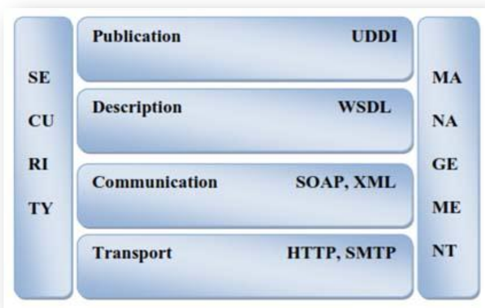
Figure 5:« Architecture des services Web »
